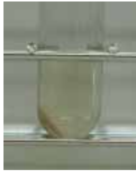
Fig. 1 Pellet forming state when using the new S55A fixed angle rotor (Rotor's cavity angle: 35°)
