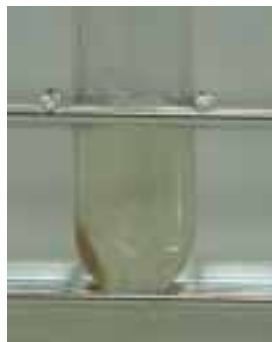
Fig. 2 Pellet forming state when using the conventional P90AT fixed angle rotor (Rotor's cavity angle: 26°)
